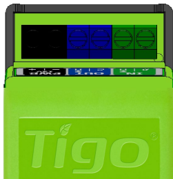
Transmitter with PST
