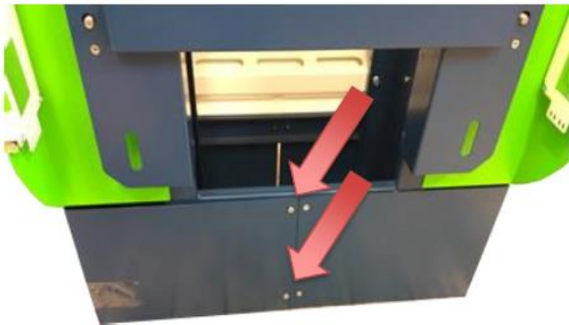
Figure 5: Screws location for the bottom cover
