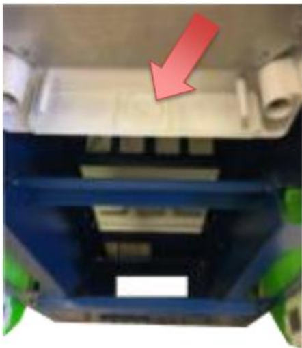
Figure 8: Hole for supply conductors
