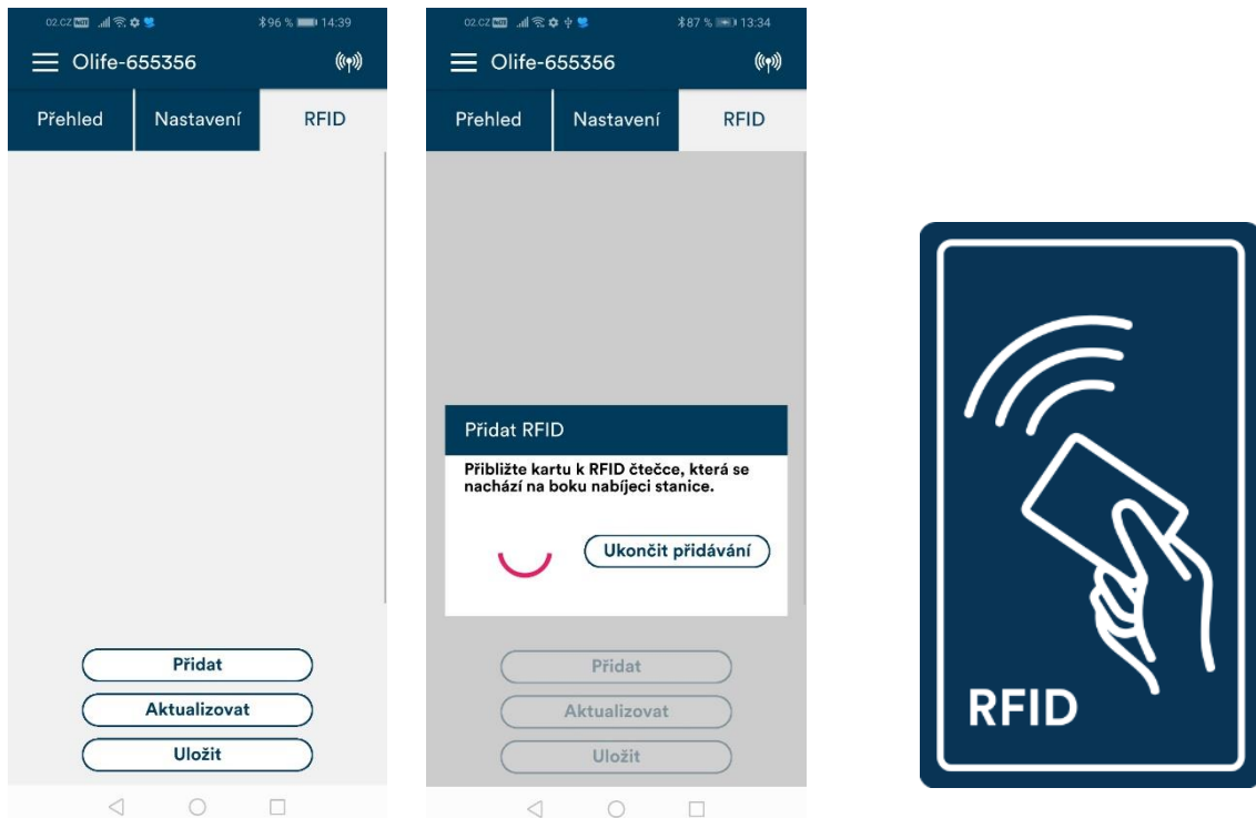
Figure6: RFID menu to add cards + a symbol on the station to which cards and chips are added
